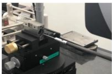
確保精度的螺帽內滾珠的調整 Ensure the precision of ball adjustment in the nut
