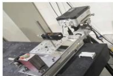
激光干涉儀檢測絕對定位精度 Laser interferometer detects the absolute accuracy of running
