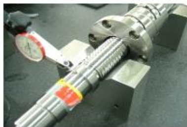
滾珠絲杆軸端檢測 Ball screw shaft end inspection
